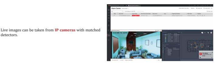
When the system is started, fire events coming from the addressable system are transmitted from Sprvsr+ Plug-In to HikCentral. The transmitted alarm is displayed in the HikCentral "Alarm Center" window.
